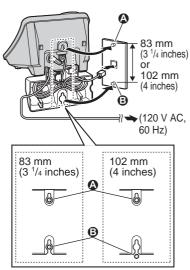
To remove the wall mounting adaptor While pushing down the lever (1), remove the adaptor (2).
