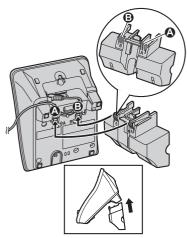
2 While pressing down the lever (1), press it in the direction of the arrow (2) until it is secure.
